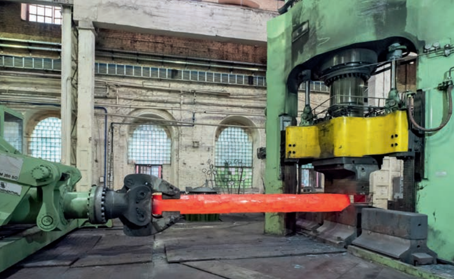
Forging and elongating of the blank guided by the manipulator
