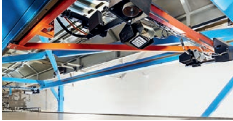
Section transfer cart
