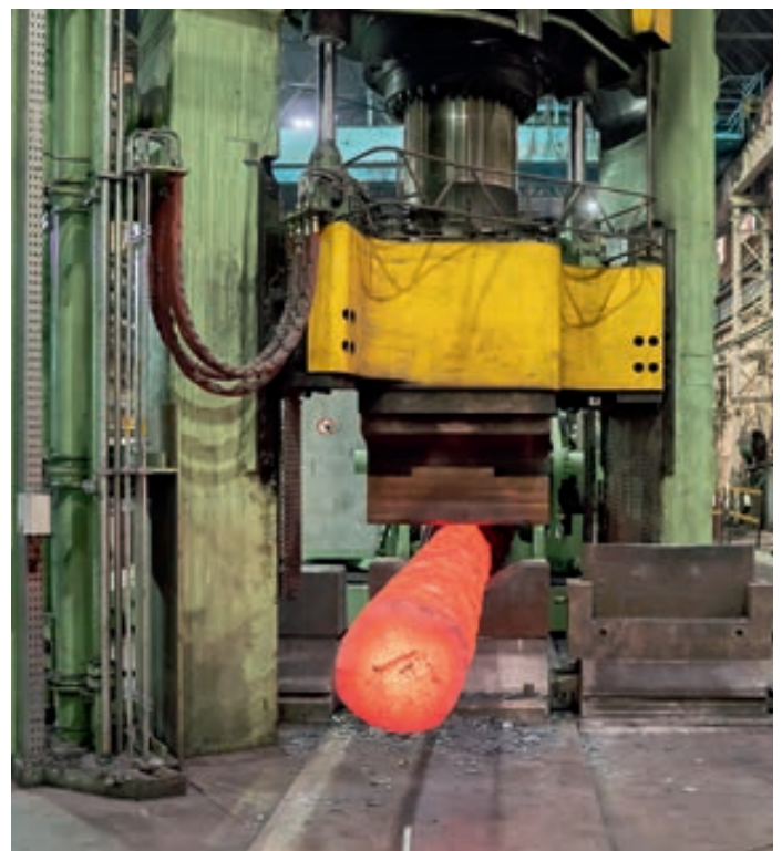
Round forging by turning the blank between press strokes
