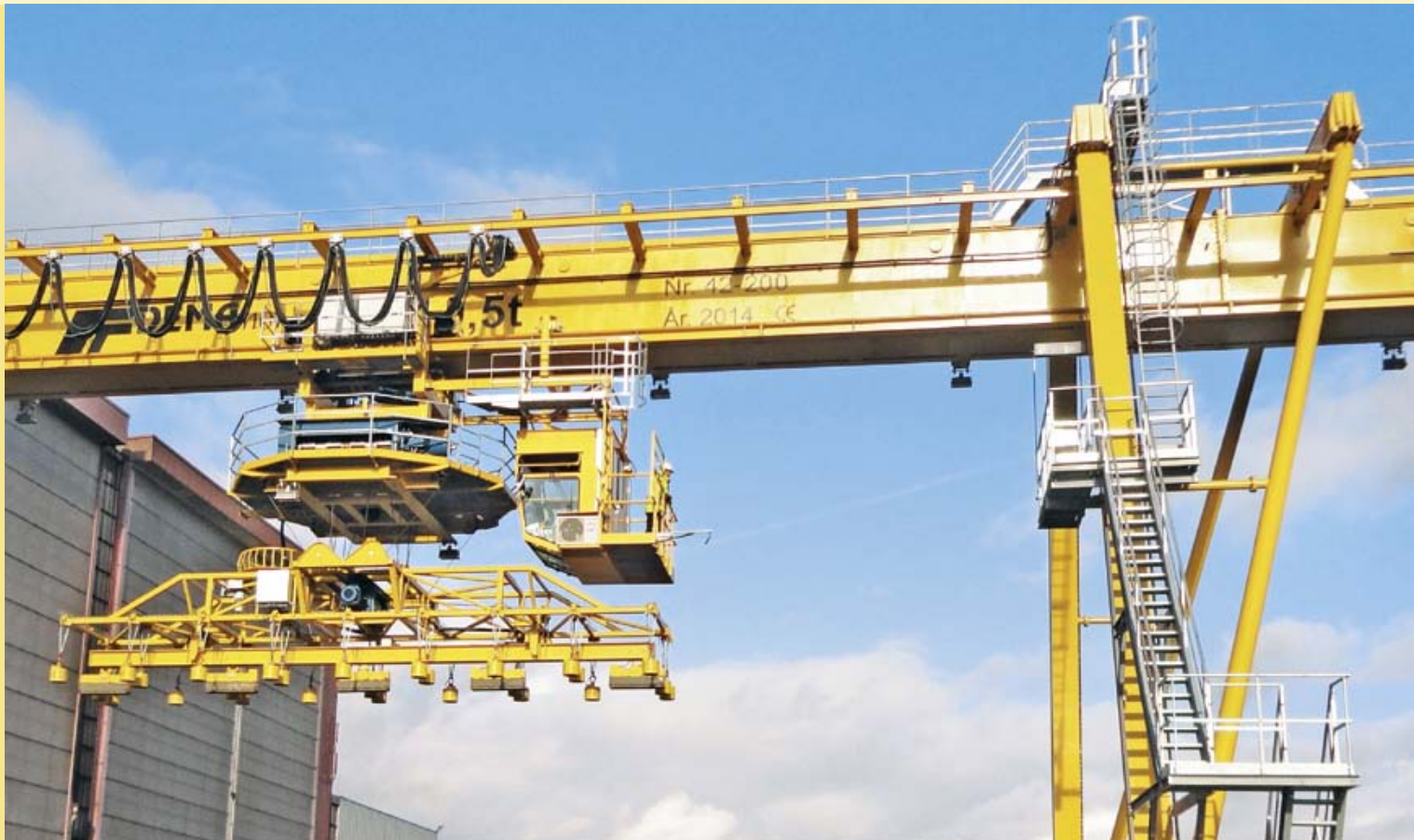
Rotating crab and magnetic crossbeam
