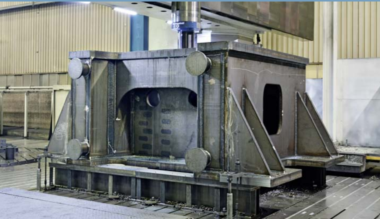
Lower beam during machining in Krefeld
