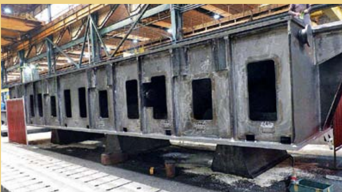
Lower beam: welded construction
