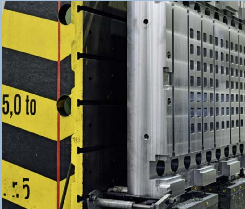
The press table during manufacturing
