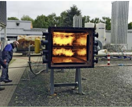
Test area for the new duct burner at the outside area of an institute in Duisburg
