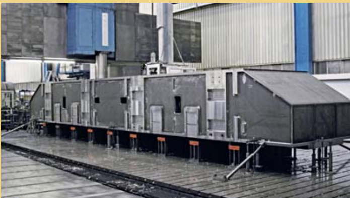
Upper beam during machining in Krefeld
