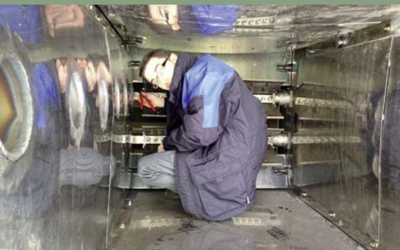
View into the burner duct, new trials with improved gas nozzles
