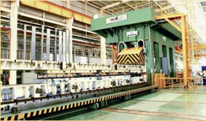
Tool shifting tables in front of the press
