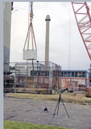
Drop test: dropping from a height of 5.20 m
