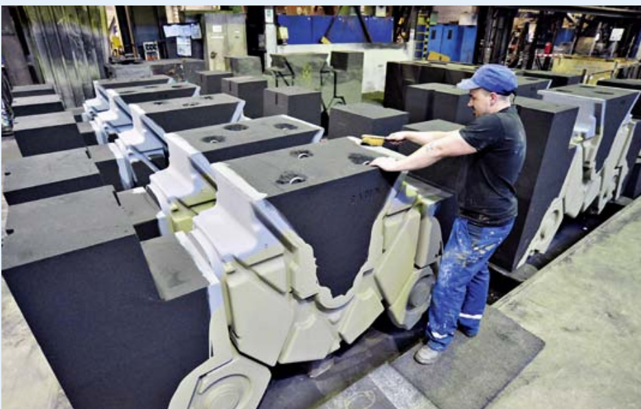
The core of the engine: finished coated cores
