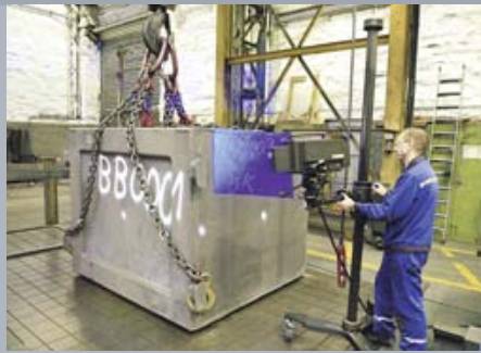
Optical 3D measurement of the new container type
