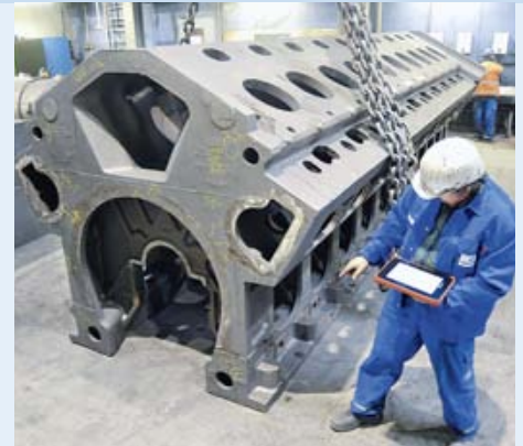
Checking the work steps already performed in the fettling shop
