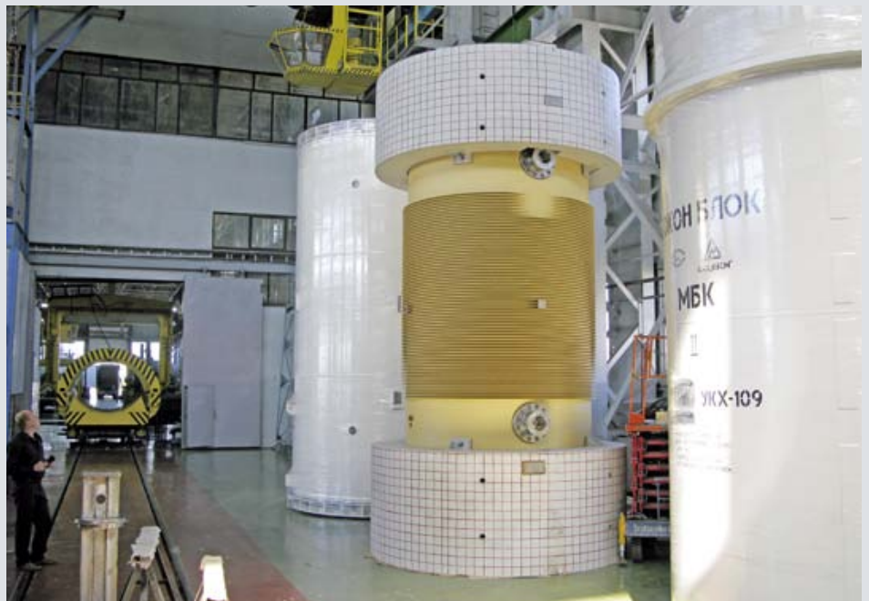
Preparation for the drop test: equipping the TUK-141 with shock absorbers at the warehouse of Siempelkamp's cooperation partner (on the right)
