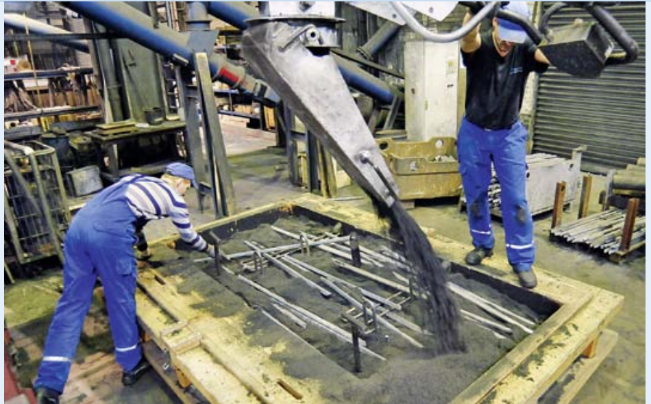
Filling quartz sand into the core box
