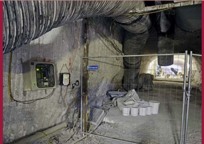
Dosimeter reader (left) at the 750 m level inside the Asse pit at the entrance of the monitoring area (Photo: Asse-GmbH)
