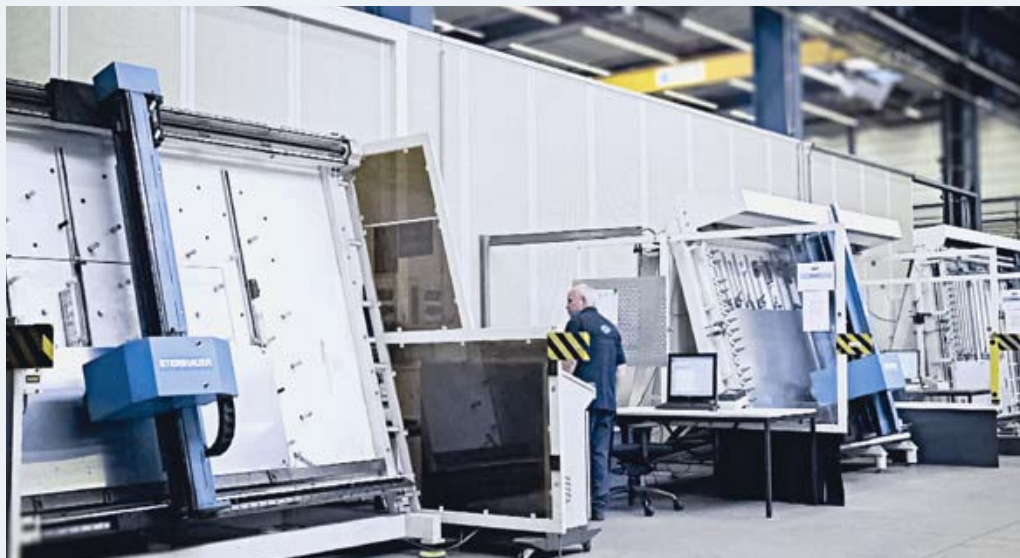
Automatic drilling machines for the mounting plates
