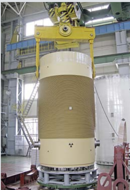
Preparation for the drop test: equipping the TUK-141 with shock absorbers at the warehouse of Siempelkamp's cooperation partner (on the right)
