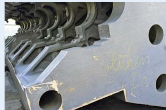
Completely machined and ready for the annealing process
