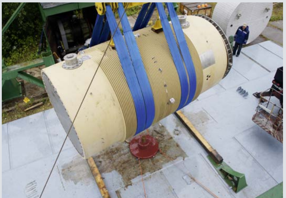
Accident scenario: impact on a steel punch of 15 cm in diameter, from a height of 1 m for subsequent leakage testing
