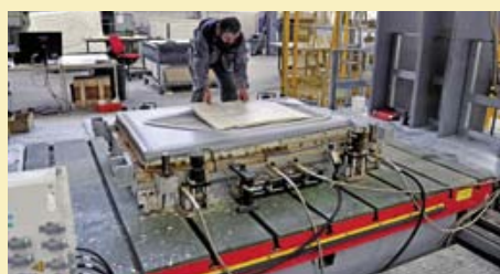
Loading fiber composite mat – test run
