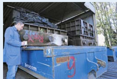
The engine block with its molding box on the cooling yard
