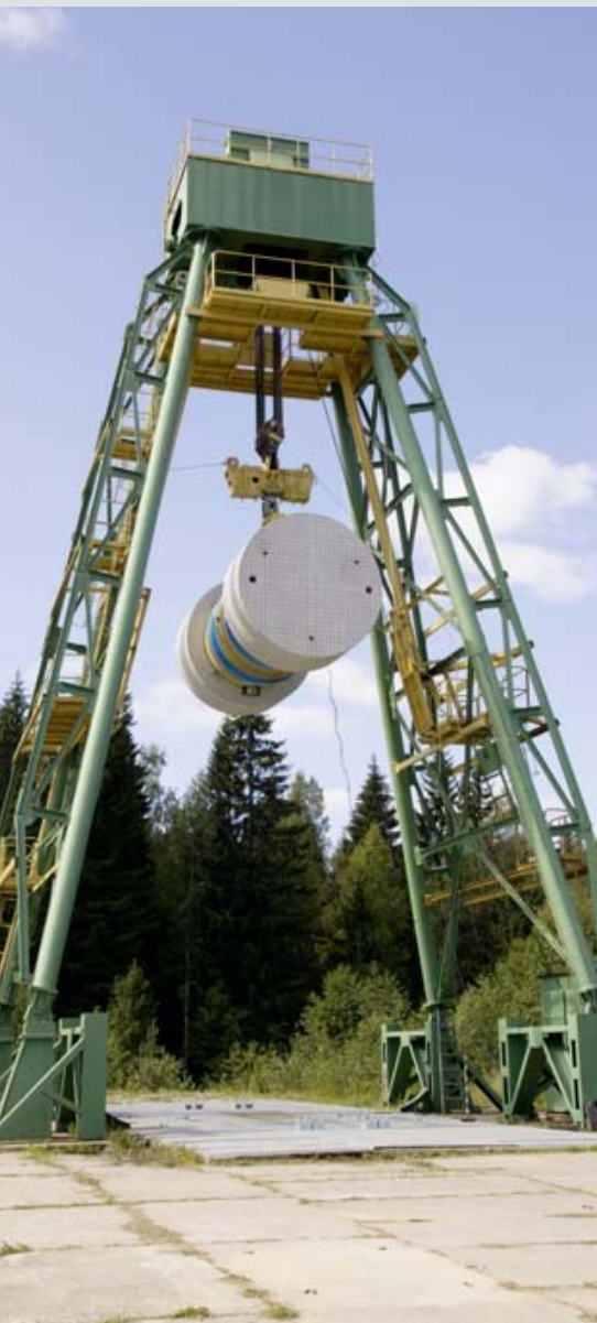
9 m drop test: crashing fall – for maximum safety
