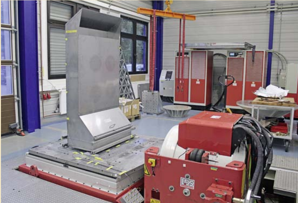
Earthquake simulation in the NIS Technical Center: fixed on a vibrating table, the reliability check of the H2-recombiners takes place
