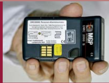
Personal alarm dosimeter: an alarm is triggered when predefined limits are exceeded
