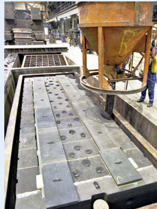
The engine block set in sand: filling of frame and cope box with quartz sand
