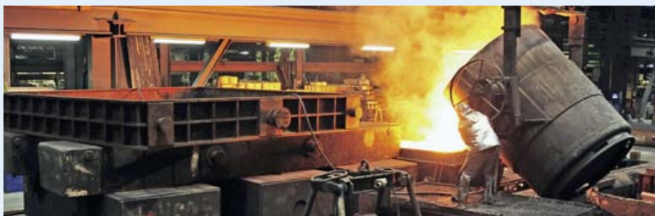
The great moment: the liquid iron for the future engine block flows into the mold
