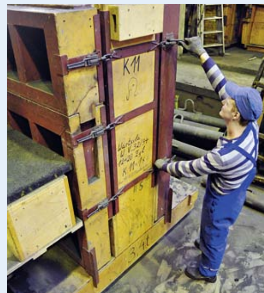
Inspection of the core box
