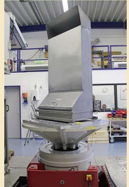
Earthquake simulation in the NIS Technical Center: fixed on a vibrating table, the reliability check of the H2-recombiners takes place
